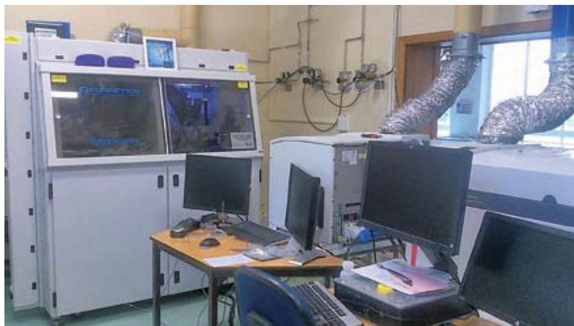
This is our other Resolution 193 nm laser-ablation system connected to the Agilent 7700 ICP-MS and used for whole-rock trace-element analysis. The laser can also be connected to the Agilent 8800 QQQ ICP-MS for high-sensitivity trace-element or U-Pb isotope measurements.
