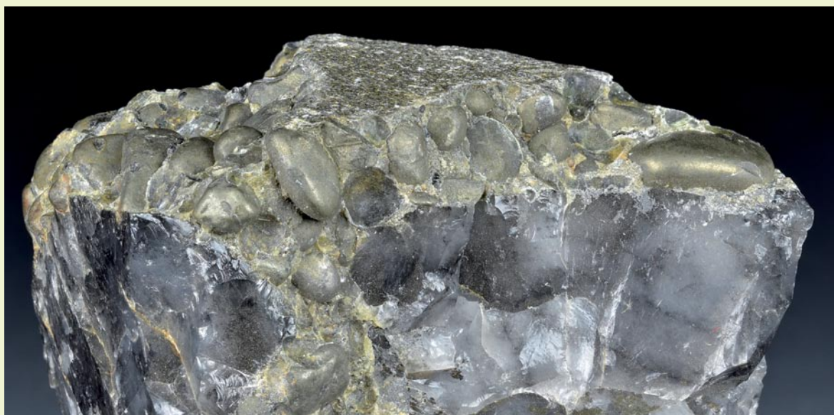
Figure 4. Layers of pyrite in the quartz pebble conglomerate reef from the Vaal Reefs gold mine, Witwatersrand goldfield. The pyrite is present as inclined layers of detrital pyrite on the foresets of cross-bedding. The 13.5 X 12 cm specimen is polished and photographed in direct reflected light to highlight the pyrite layers. Bruce Cairncross specimen and photo.
