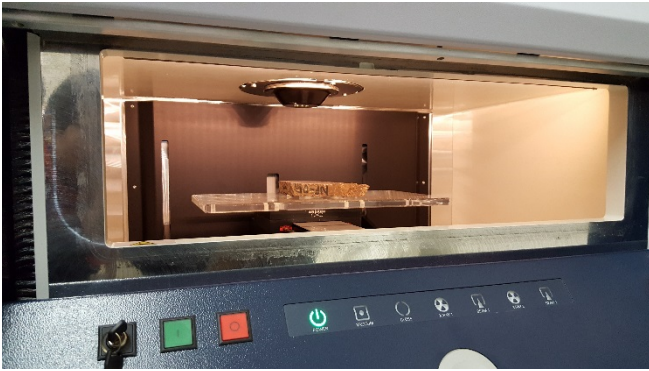
Sample block placed in the chamber of the micro-XRF instrument.
