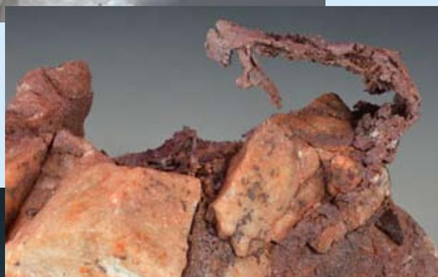
*Flattened platelets of copper partially imbedded in quartz. Field of view is 4 cm. Klein Aub Mine, Namibia. (Specimen and photo: Bruce Cairncross)*
