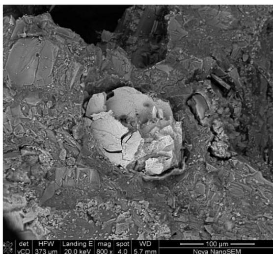
Curved-faced brochantite crystals may be a sign of cyclical erosion and deposition. A thin layer of copper sulphate connects the cavity to the matte source and the slag surface. BSE image.
