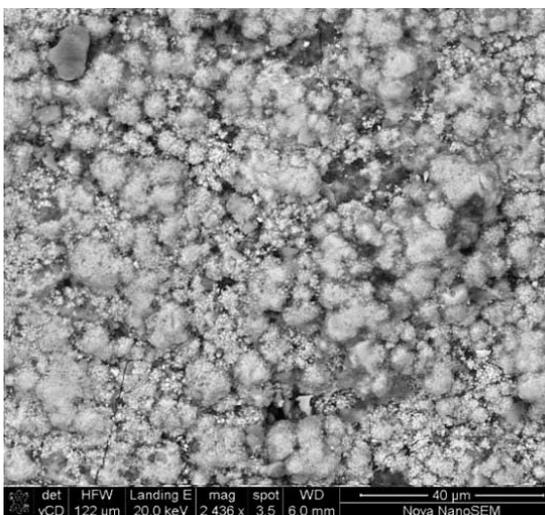
*Amorphous copper chloride, probably atacamite, or a partially hydrated form. This forms as green crusts on Jubilee slag where there is groundwater contact. BSE image.*
