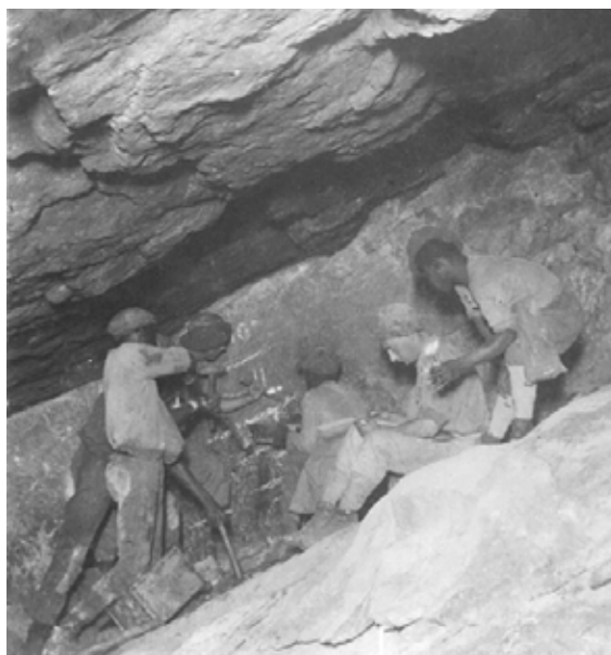
Sampling the reef at Crown Mines. Sections have been marked off using chalk to delineate the sample intervals. The miner (geologist?) can be seen hammering with a steel chisel while the labourer sits holding a container to catch the fragments. A second miner sits and records the sampling.
