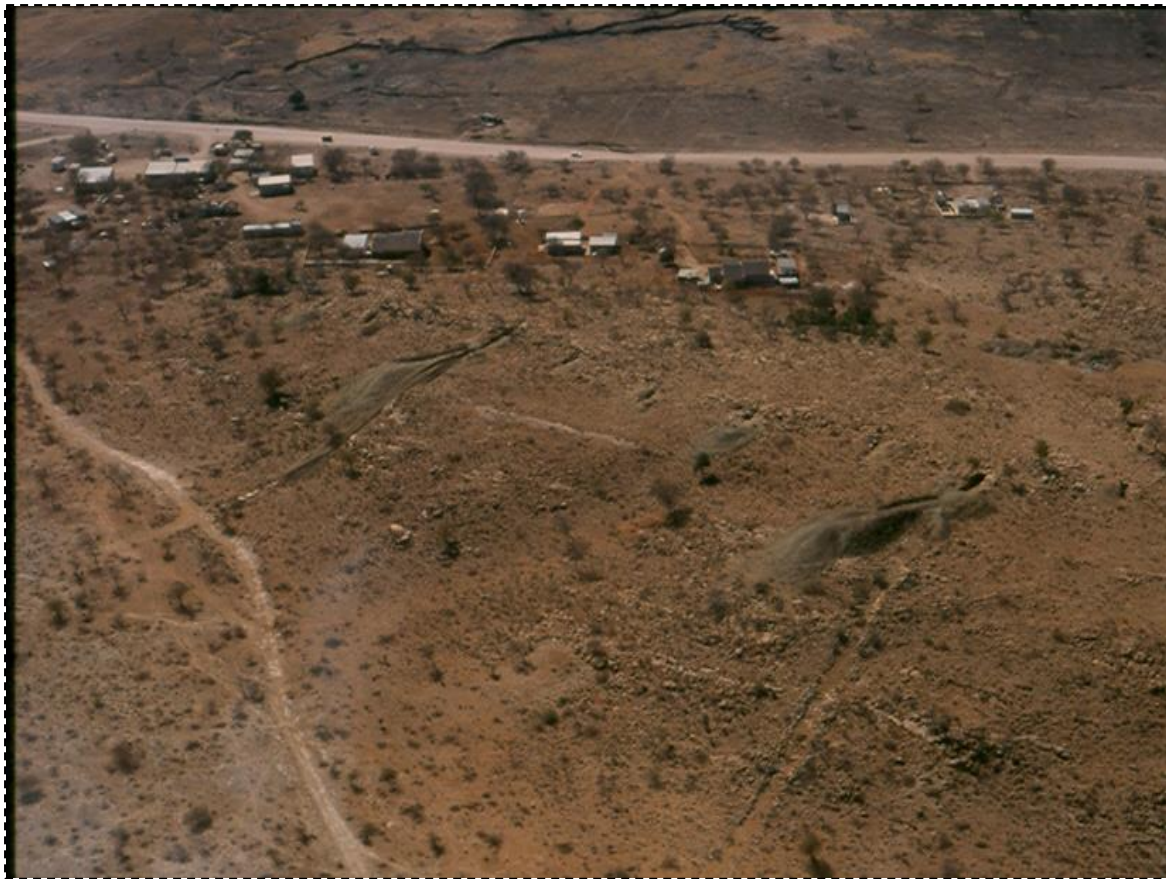
Aerial view of the historical workings on the Merensky Reef, Winnaarshoek. View looking approximately west with the line of trenches on the east facing slopes marking the outcrop of the reef
