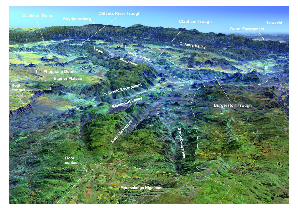
A three-dimensional satellite image (two times vertical exaggeration) of part of the Eastern Limb looking north from Die Berg with the deeply-incised valleys of the Groot and Klein Dwarsrivers in the foreground. The irregularity of the basal contact, particularly between the towns of Steelpoort (S) and Burgersfort (B) contrasts with the planar nature of the roof. The platinum discoveries were made in the Motse Valley and subsidiary tributaries that occupy a broad valley at the foot of the Bushveld Escarpment. (Landsat 7 image for the year 2000 sourced from the University of Maryland Global Land Cover Facility and processed by Philip Eales of Planetary Visions)
