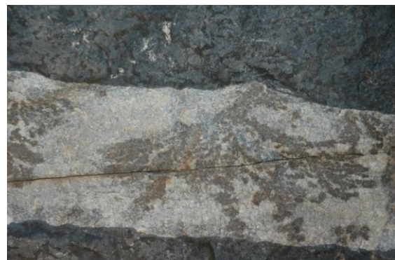
Dendritic mottle (oikocrysts) of pyroxene within a thin layer of anorthosite intercalated between two chromitite layers
