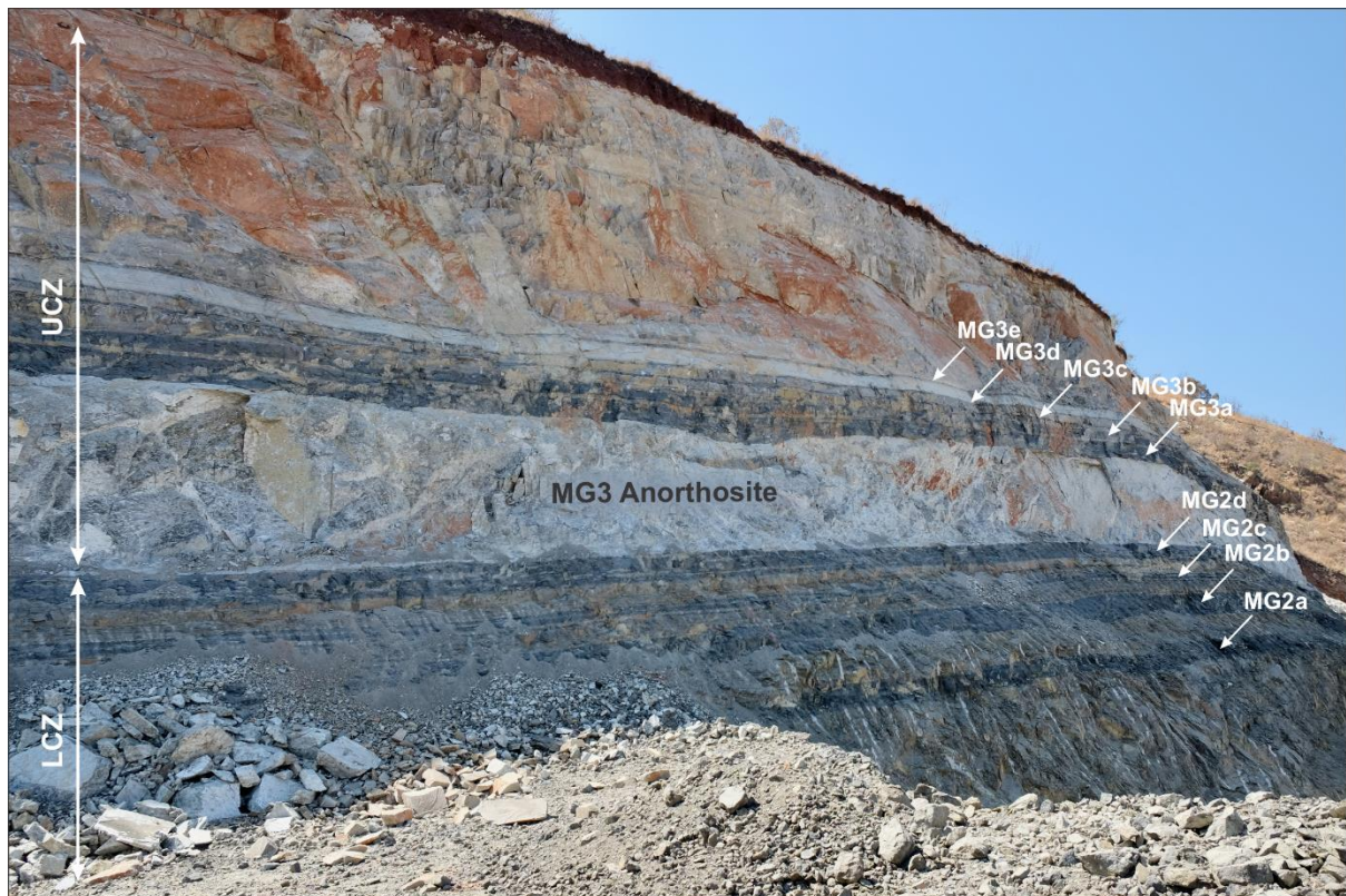
The multiple nature of the MG2 and MG3 chromitites as seen in the De Grooteboom open pit. The MG2-ad seams occur below the MG3 Anorthosite; the MG3a-c seams are located either above the anorthosite or, as in this case, in the upper part of the anorthosite
