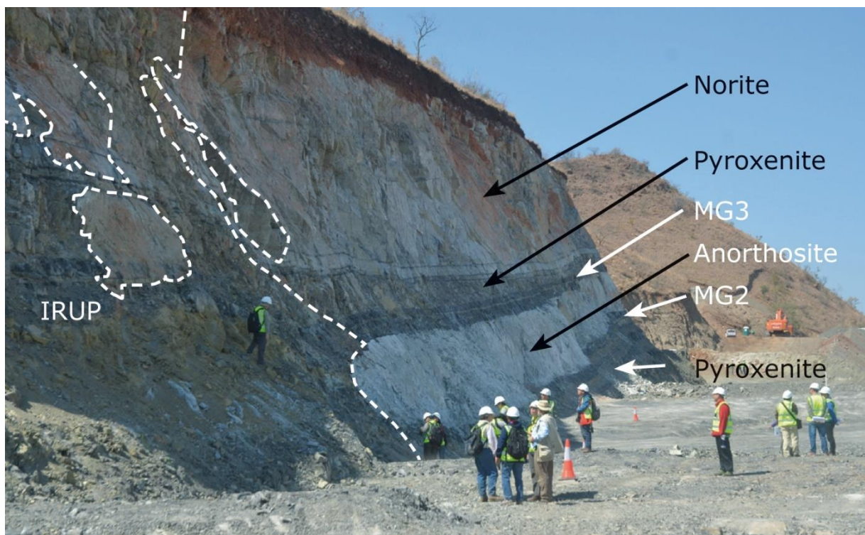
An irregular body of IRUP (dark) penetrates downward and partially replaces a layered sequence of norite, feldspathic orthopyroxenite and chromitite, open pit at the De Grooteboom mine
