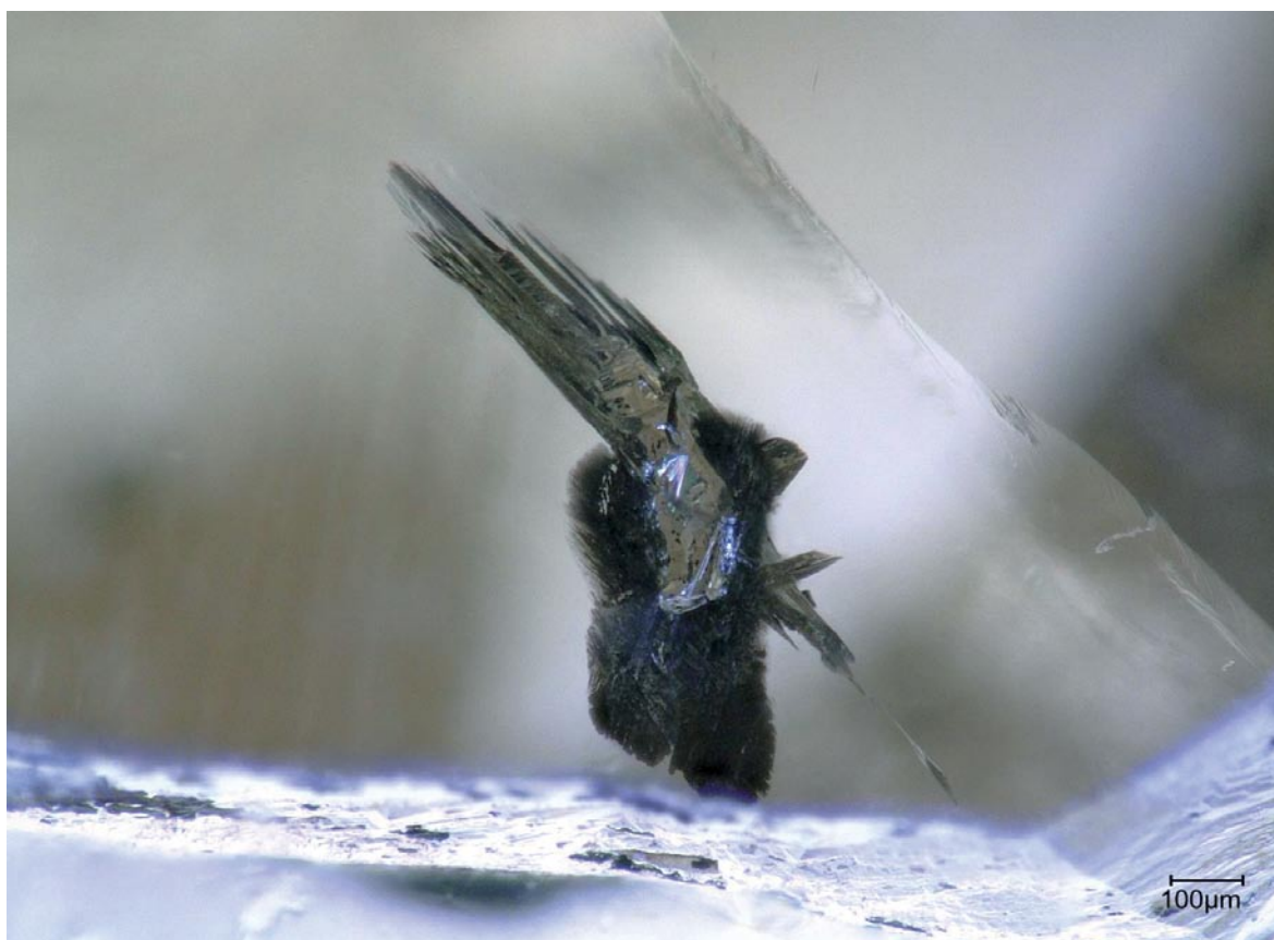
Sulphide inclusions still trapped in the Zimmi diamonds. Sulphides are silver-grey in appearance and are surrounded by blackened fracture systems. These fractures develop during kimberlite ascent because the sulphides expand more than the diamond. Photos by Karen Smit/GIA.
