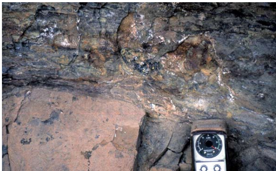
Very high-grade uranium mineralisation in Karoo sandstone on cliffs along the Great Escarpment east of Sutherland. The hand-held scintillometer is off-scale! Similar high concentrations of uranium caused natural nuclear reactions to occur at the Oklo deposit.
