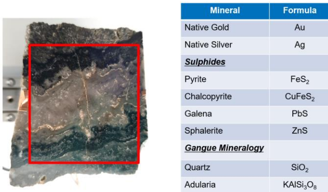
Figure 2. Gold-bearing epithermal sample from the Karangahake deposit, New Zealand. The sample is approximately 5 cm in width. The inset table lists the relevant minerals and elements of interest. The sample is carbon coated as both X-ray and electron analyses will be performed.
