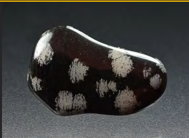
"Snowflake" obsidian. A small 3.2 cm tumbled and polished specimen. The "snowflakes" are cristobalite, formed during the partial crystallization of the volcanic glass – see https://www.mindat.org/min-8520.html Black Spring, Black Rock Desert, Millard County, Utah, USA.
