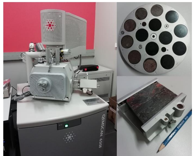
Figure 1. High resolution FEG QEMSCAN at the Centre for Minerals Research, University of Cape Town (left), standard sample holder containing 30 mm polished sections (top right), rough rock holder with ~70x70 mm polished rock slab (bottom right)
