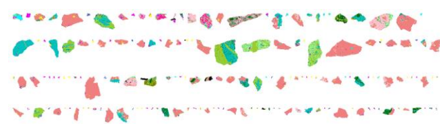
Figure 2. False-colour particle map from a sample from the Bushveld Complex UG2 Reef.
