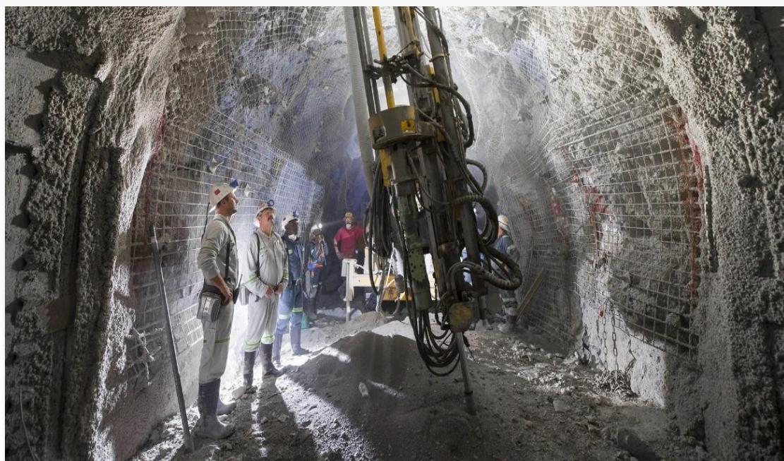
Long-hole drilling rig aligned for ring drilling to develop a draw bell at C-Cut 839L
