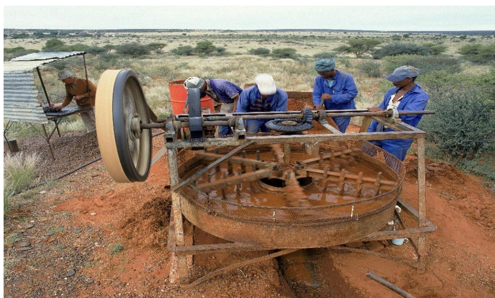
Rotary pan and sorting table for processing and recovering diamonds, Brakfontein, MOR (1998)
